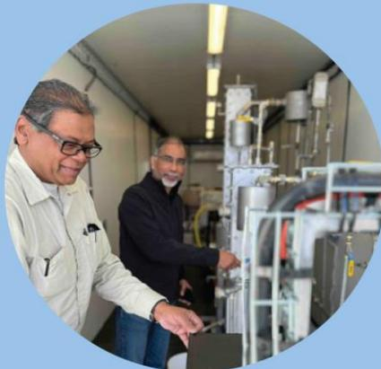
Sample demonstration plant (SPD) producing lithium carbonate from fresh brine, producing at 1 tpa
