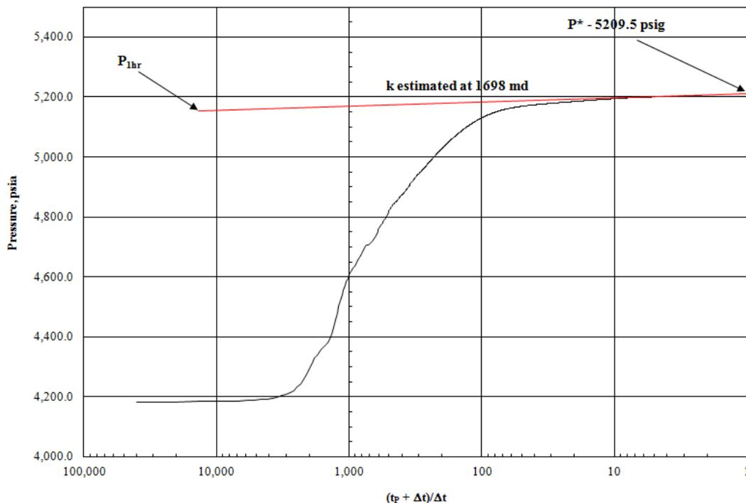
Figure 2: A plot of the Horner Analysis of the flow and build up test for Long Canyon No 2 well.
