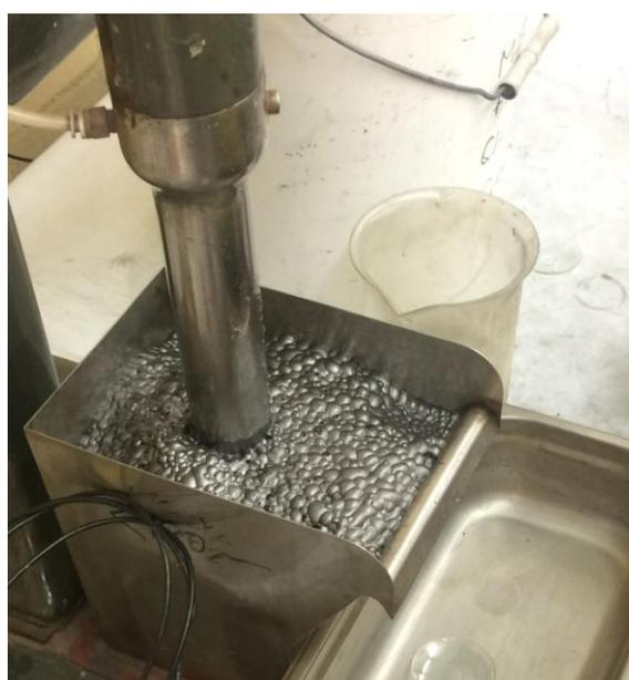
Photo 1: Flotation test
